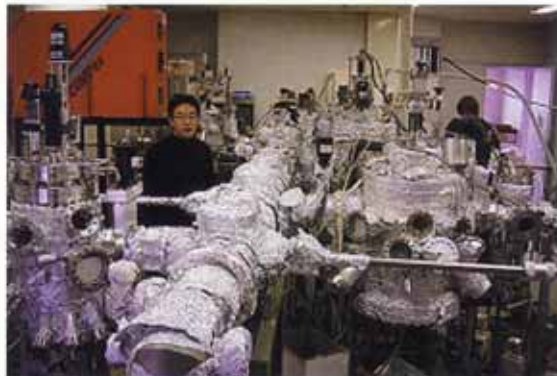
Fig. 2 Multi-chamber MBE system for epitaxial growth of semiconductor films on metal substrates.
